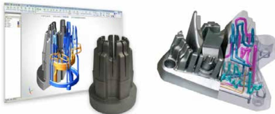
Traditionally lines are added by drilling holes and either making side intersecting holes and plugging them or not being able to cool some of these areas at all. With conformal cooling technology companies can now decrease cycle times of the parts, increase tooling life of the mold and reduce scrap. This is a new process - we have many studies that show the substantial cost saving benefits and better part production with the use of conformal cooling technology.
